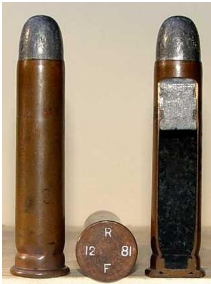
Figure 5. An external view left, and internal view right, of a .45-70-405, Benét-primed center-fire cartridge. The center picture shows the “R F 12 81” headstamp on the bottom of the copper cartridge case. The headstamp means that this cartridge is intended to be fired in a rifle (“R”), and that it was manufactured by Frankford Arsenal (“F”) in December of 1881 (“12 81”). If this was a .45-55-405 carbine cartridge, there would be a headstamp letter “C,” instead of an “R.” Picture from Salute Targets, https://www.salutetargets.com/blog/article/All+American+Big+Bore+Caliber+-+My+Fifty+Years+with+the+.45-70 . Accessed August 2022.
