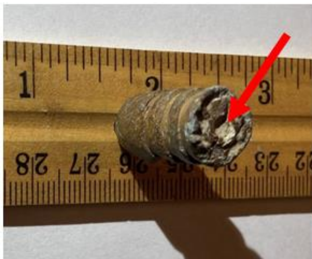
Figure 4. The red arrow points to the dished cavity on the base of the bullet. The cavity has a diameter of approximately 0.130 inches. The cavity depth, which appears to be partially filled with compacted foreign material and oxidization, is 0.055 inches. Photo by author.
